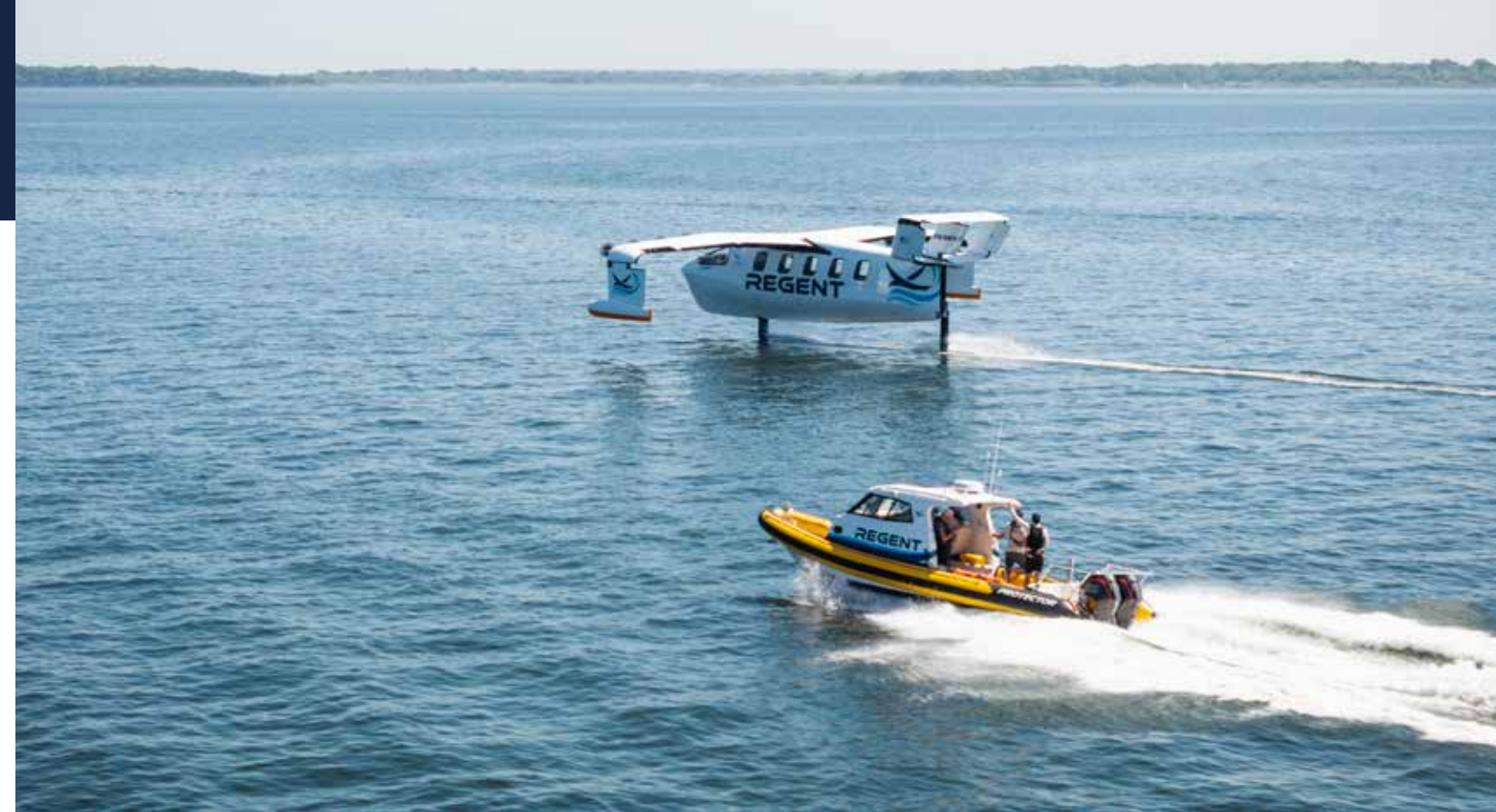
Viceroy is REGENT's flagship Seaglider vessel, a wing-in-ground-effect craft that flies just above the water's surface
